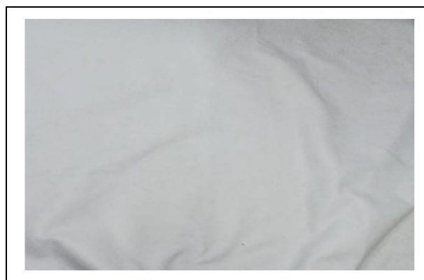
Fig. 2: Non-woven polypropylene geotextile layer
