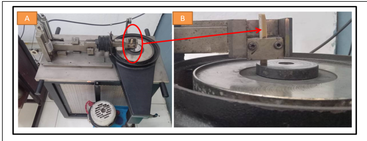
Fig. 1: Pin-on-disc (a) machine setup and (b) enlarged view of sample position
