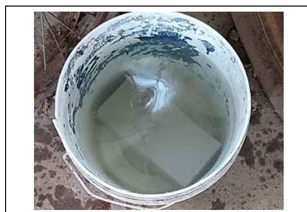
Fig. 8: Water Absorption Test
