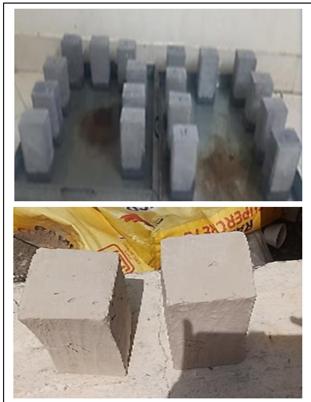
Fig. 9: Water absorption test
