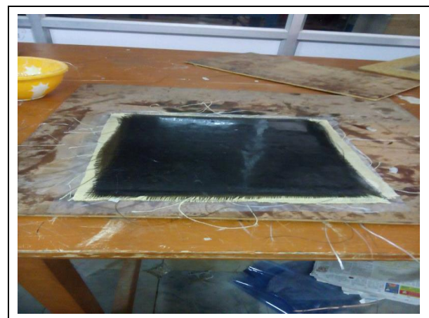
Fig. 8: Completed extended unidirectional TiO 2 with natural fiber composites for NNF/EP
