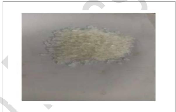
Fig. 3: Silica gel beads used as moisture-retention additive
