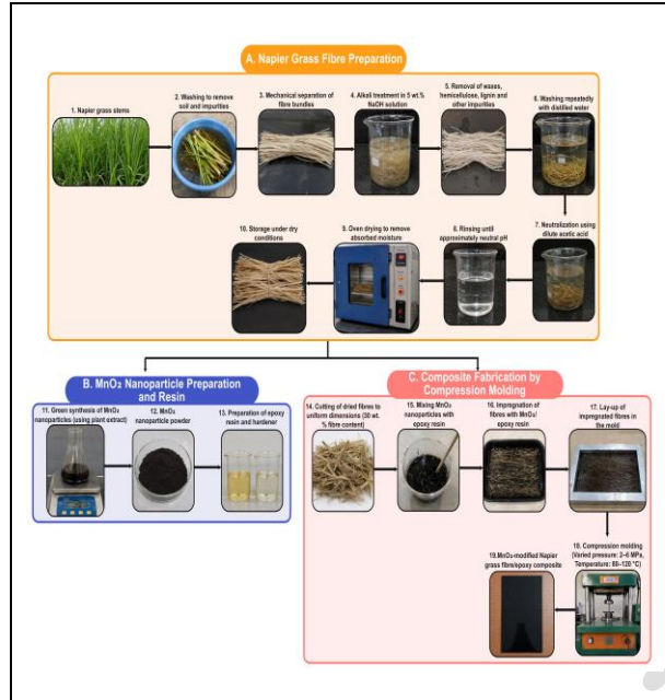
Fig. 3: Fabrication sequence of green-synthesized \text{MnO}_2 -modified Napier grass fibre/epoxy composites
