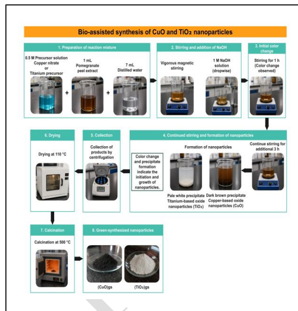
Fig. 1: Bio-assisted synthesis of CuO and TiO 2 NPs
