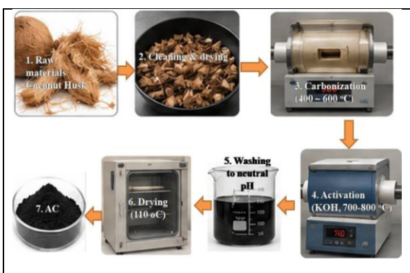
Fig. 1b: Preparation of activated carbon (AC)
