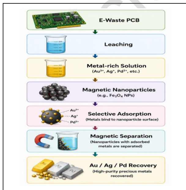
Fig. 3: Nanotechnology-based precious metal recovery mechanism
