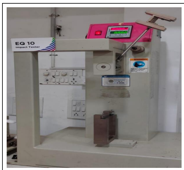
Fig. 2: Impact testing machine setup (Izod Test)
