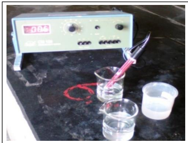
Fig. 5: Conductance measurement of plant extracts
