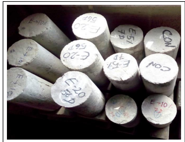
Fig. 7: Split tensile strength test
