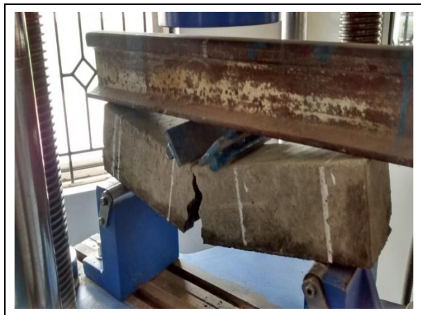
Fig. 8: Modulus of Rupture test
