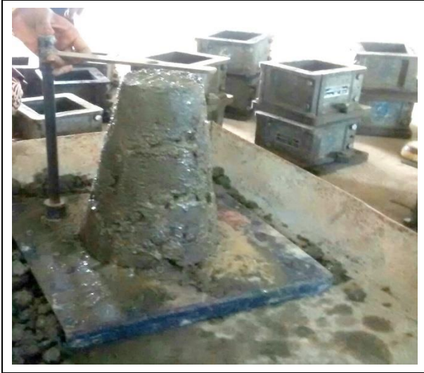
Fig. 6: Slump test on fresh concrete
