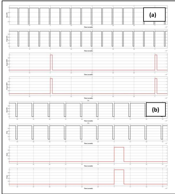
Fig. 6: Pulse generator waveform for (a) 2 \mu\text{s} at 10 \Omega (b) 6 \mu\text{s} at 10 \Omega
