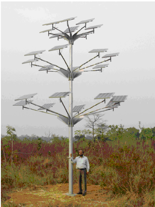
Fig.7: Prototype of Solar Power Tree Capacity 2 KWh (Area 3 Sq. Ft)
