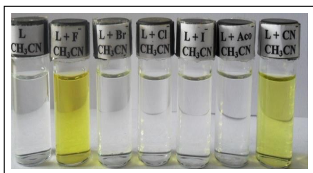
Fig. 7: Color changes of sensor (L=L1) ( 5.0 \times 10^{-5} M) in \text{CH}_3\text{CN} before and after addition of 0.2 equiv of representative anions (from left to right: L, L+F, L+Br, L+Cl, L+I, L+Aco, L+CN)
