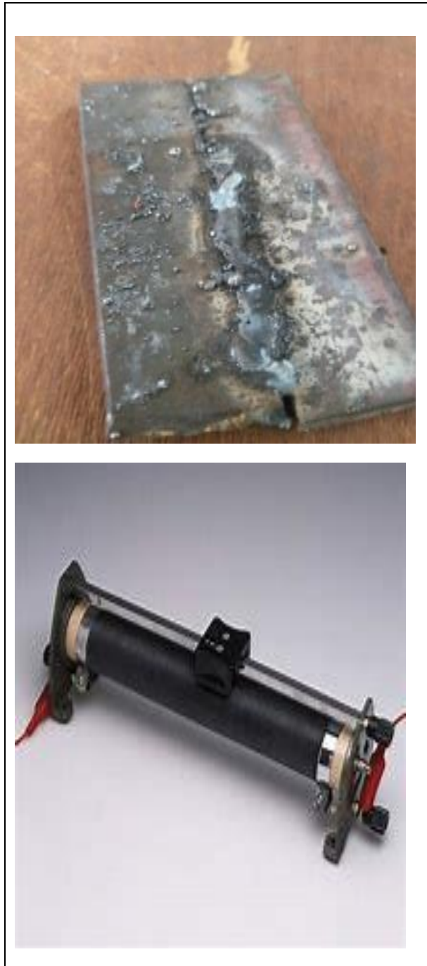
Fig. 2: The chip (Mild steel) and Rheostat
