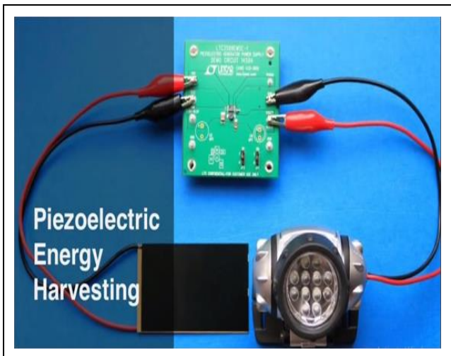
Fig. 10: Hardware implementation Piezoelectric-driven Supercapacitor setup.
