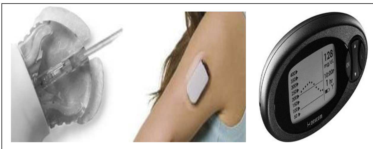
Fig. 13: Continuous Glucose Monitoring (CGM) Sensor, Receiver and Transmitter
