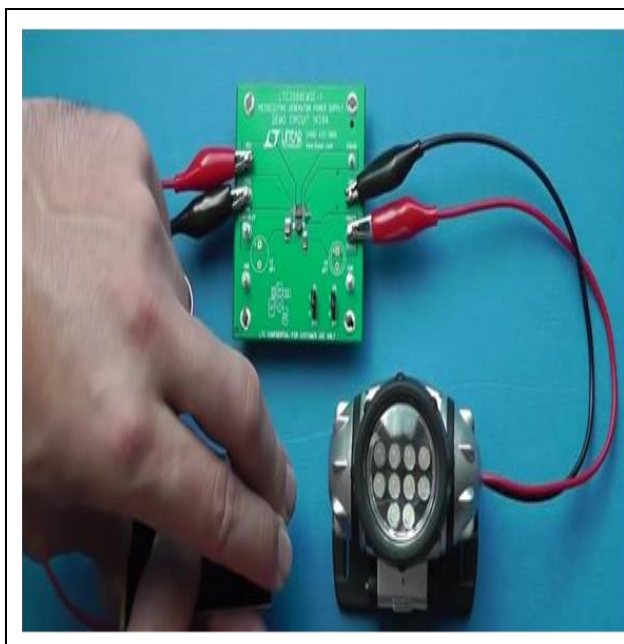
Fig. 11: Piezoelectric-driven charging Supercapacitor
