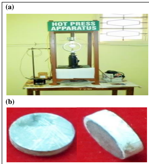
Fig. 7: (a) Hot press apparatus, (b) Pellets made by hotpressing.
