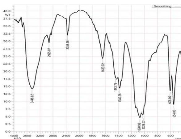
Fig. 2: FTIR spectrum of Mg-Hap
