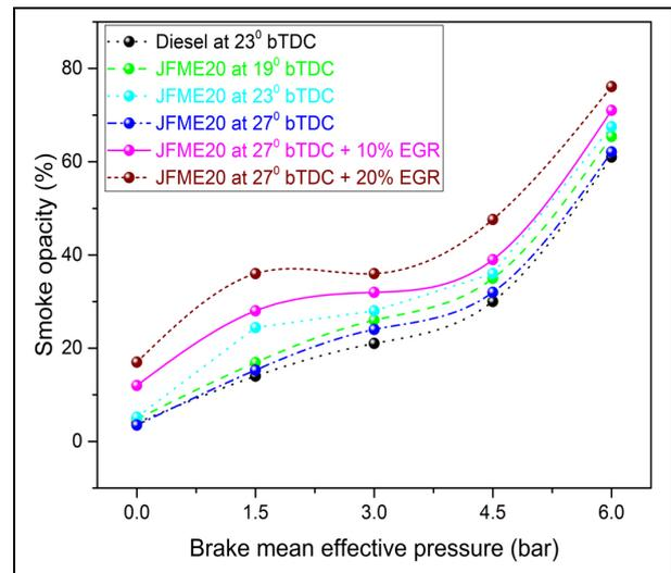
Fig. 9: Variation of smoke opacity with BMEP
