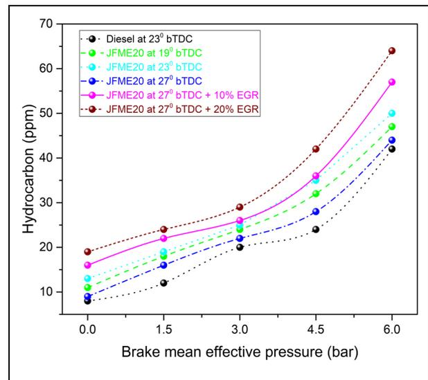
Fig. 6: Variation in HC emissions with engine load
