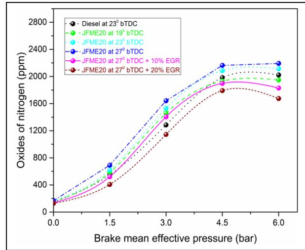
Fig. 8: Changes in NO<sub>x</sub> emissions according to engine load
