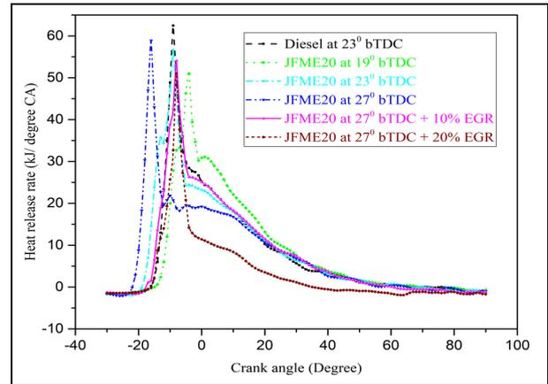
**Fig. 11: HRR variation with engine crank angle**
