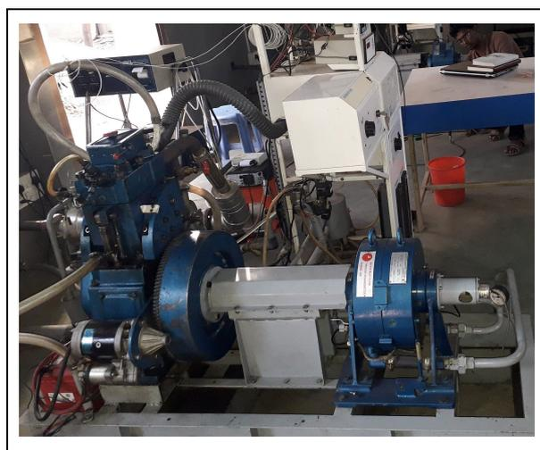
**Fig. 3: Experimental setup of diesel engine**
