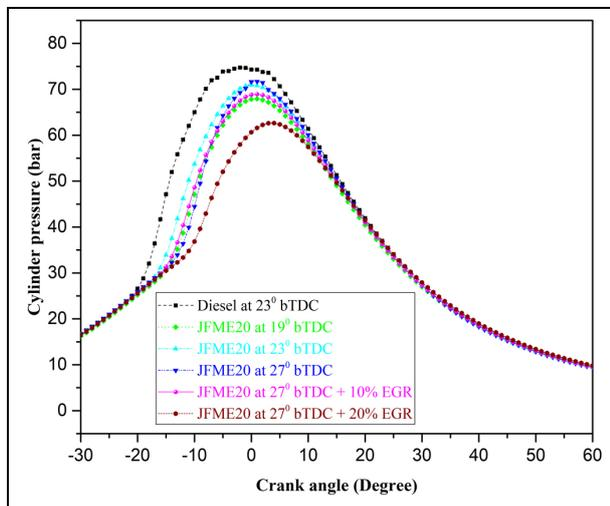
**Fig. 10: Cylinder pressure variation at various crank degrees**
