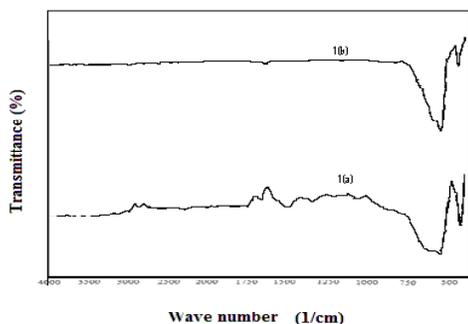
**Fig 1(a & b) FT-IR spectra of Magnesium ferrite samples sintered at (a) 130<sup>o</sup>C (b) 600<sup>o</sup>C**
