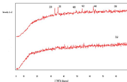
**Fig 2(a & b) XRD analysis of Magnesium ferrite sample sintered at (a) 130<sup>o</sup>C (b) 600<sup>o</sup>C**
