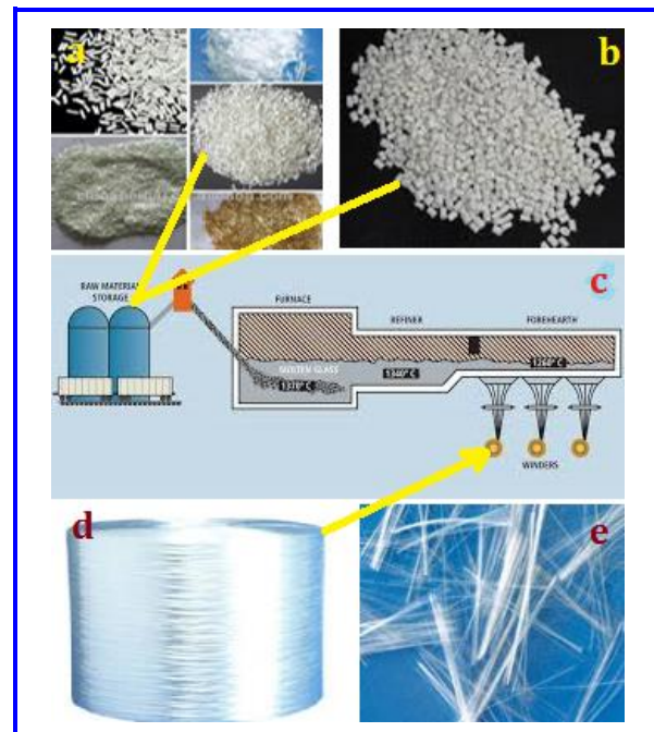
Fig. 1: Processing of glass fiber (a-b) raw materials (c) processing technique (d-e) glass fiber roll and Glass fibers.
