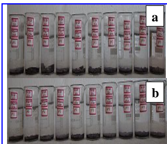
Photo 5: Effect of pH on the photocatalytic degradation of textile effluent at 120 minutes [textile effluent = 3%, (a)= \text{CaAl}_2\text{O}_4\text{-I} , (b)= \text{CaAl}_2\text{O}_4\text{-II} ,]
