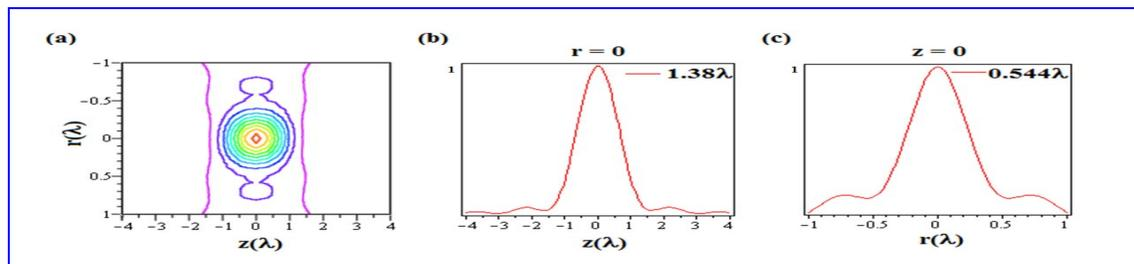
Fig. 2: Total electric field intensity distribution (a). Contour profile, (b). normalized two dimensional intensity distribution at  $r = 0$  and (c). normalized two dimensional intensity distribution at  $z = 0$
