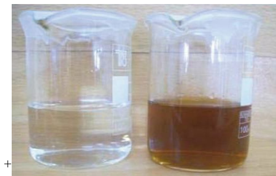
Fig 2: Picture of aqueous solution of 1mM Silver nitrate with putranjiva roxyburghii wall leaf extract before adding the leaf extract and after addition of leaf broth.
