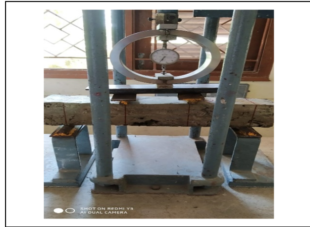
Fig. 7: Flexural strength test set up
