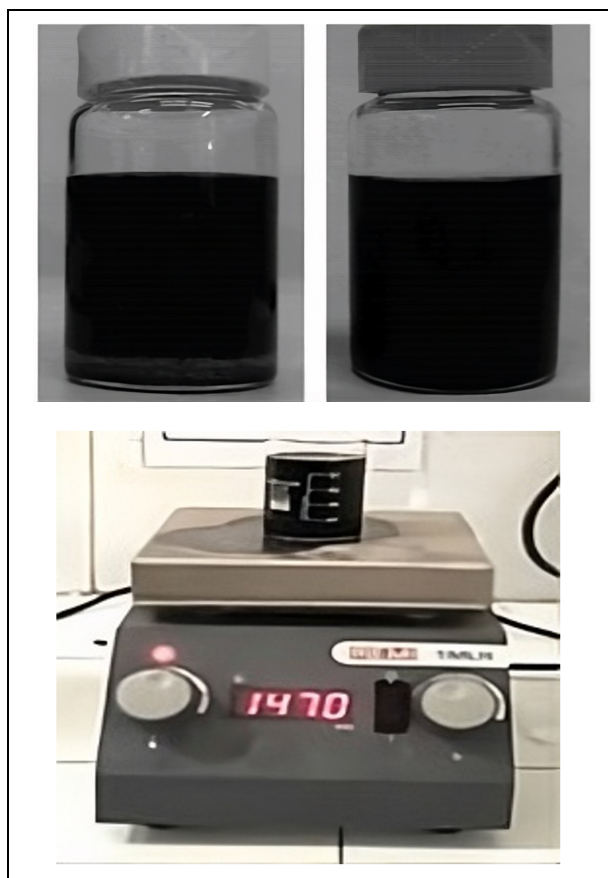
Fig. 1: MWCNT with polycarboxylate ether
