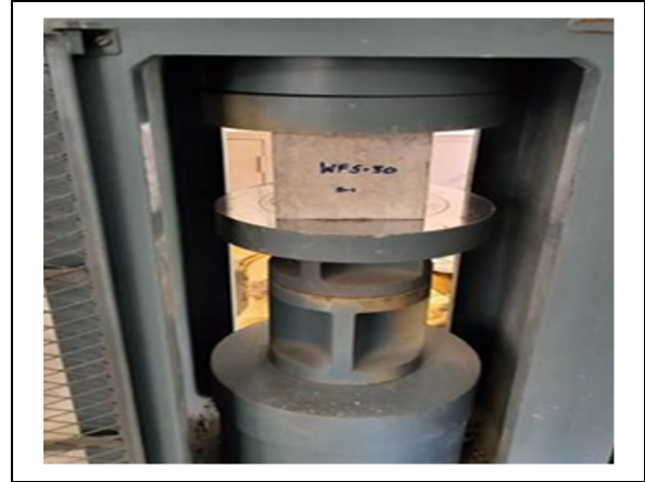
Fig. 7: Compressive strength test on a 150 mm concrete cube using a CTM
