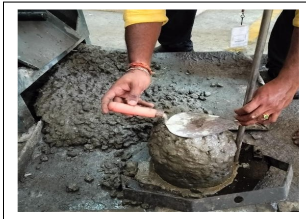
Fig. 6: Slump test setup for workability evaluation of fresh concrete
