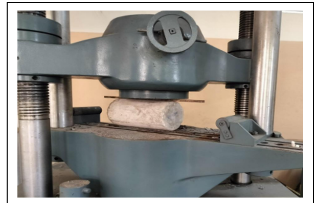
Fig. 8: Split tensile strength test setup for a 150 mm × 300 mm concrete cylinder
