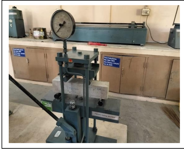
Fig. 9: Flexural strength test setup for 100 mm × 100 mm × 500 mm concrete prism
