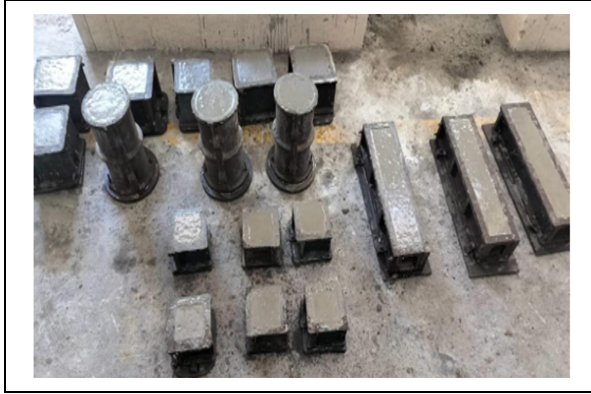
Fig. 5: Concrete specimens (cubes, cylinders, and prisms) for mechanical strength testing
