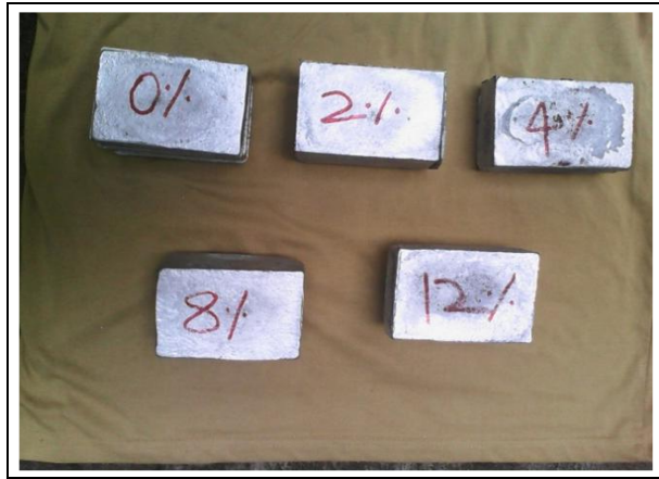
Fig. 4: Synthesized composites of AA6061 with nano-SiO 2
