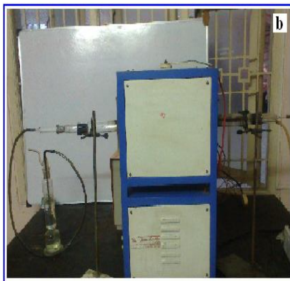
Fig. 3b: Snapshot of setup home-made experimental spray-pyrolysis set-up used for the synthesis of BS-carbon nanotubes.
