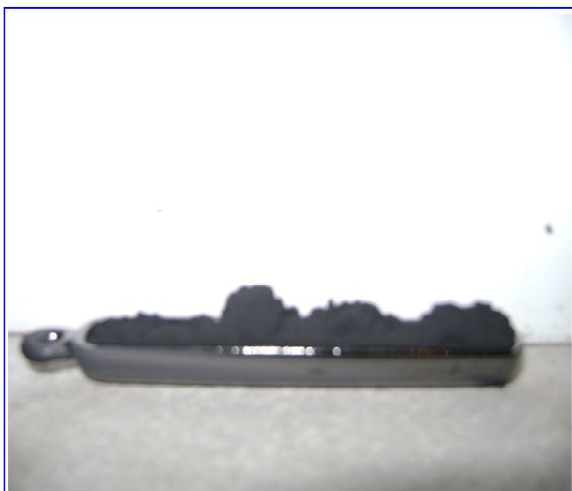
Fig. 1: The snap shot of CNTs grown over catalyst support kept in a quartz boat
