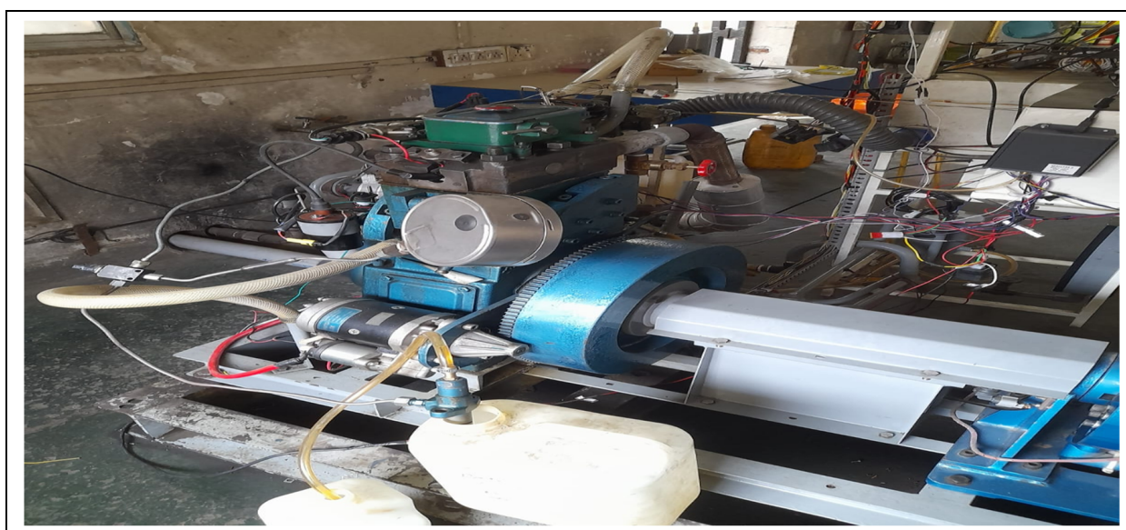
Fig. 6: Non-road engine test rig with electrical dynamometer
