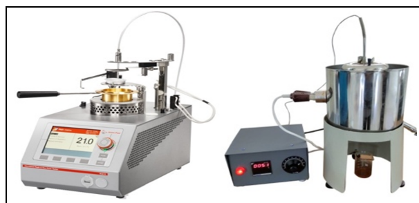
Fig. 3: Experimental setup for measuring (a) flash point/fire point and (b) viscosity
