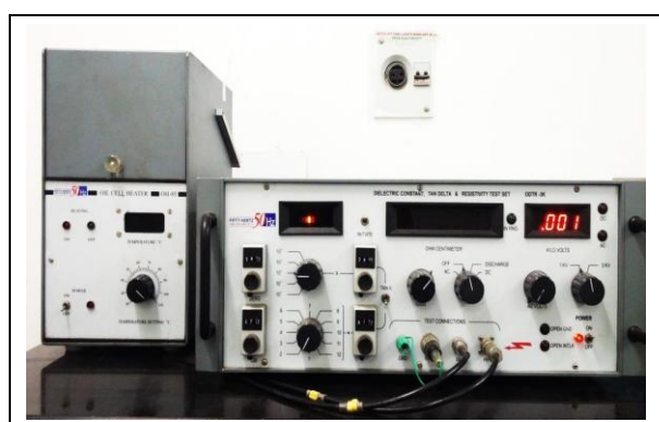
Fig. 2: Setup for measurement of dielectric constant, loss factor and volume resistivity
