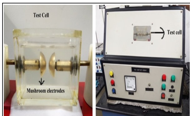
Fig. 4: BDV test setup with electrode configuration
