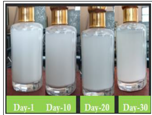
Fig. 9: Photographic evidence of the stability of the Al 2 O 3 -ethanol nanofluid over the observation period
