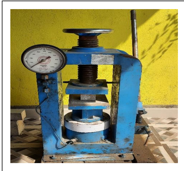
Fig.3: Compressive strength testing of nano-modified geopolymer mortar specimens
