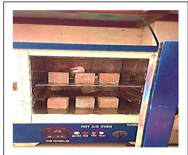
Fig. 4: Oven-dried specimens before water absorption test
