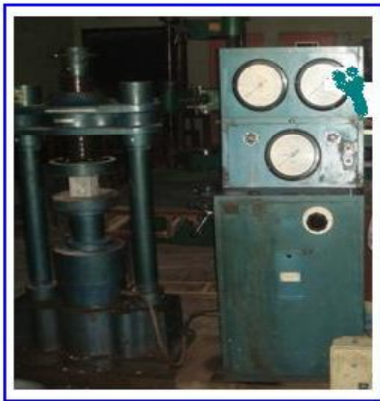
Fig. 1: Test set up for compressive strength test of concrete
