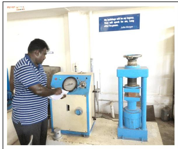
Fig. 7: Compressive strength test for IGMB prism
