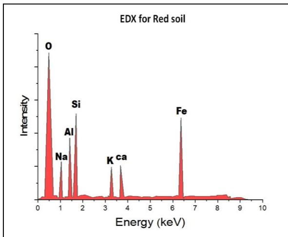
Fig. 13: EDX analysis of red soil
