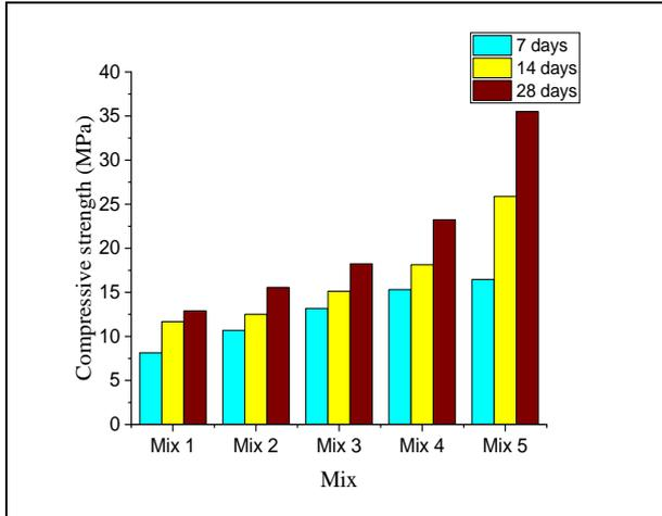
**Fig. 8: Compressive strength test for IGBM Prism results**
