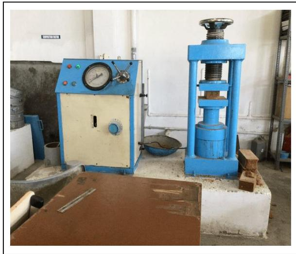
Fig. 5: Compressive strength analysis test
