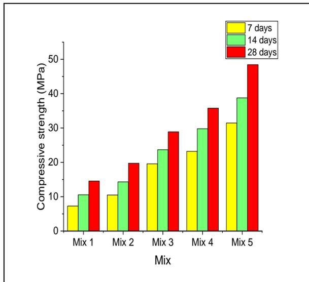
Fig. 6: Compressive Strength test results
