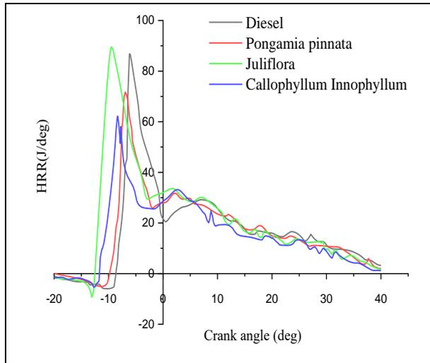
Fig. 16: Heat release rate with crank angle (deg)
