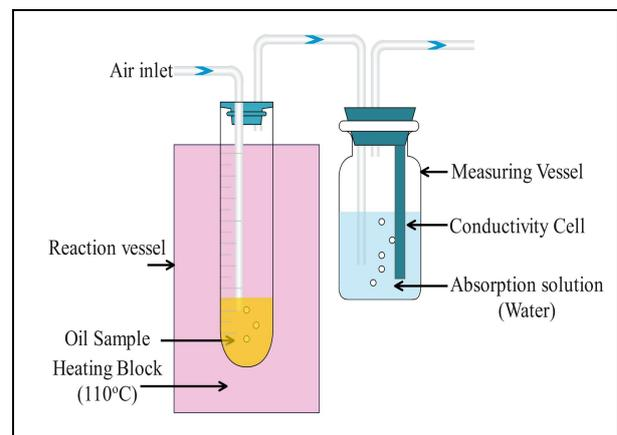
**Fig. 4: Schematic view of rancimat apparatus**
