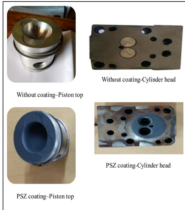
**Fig. 2: Plasma spraying process applied to engine components for LHR modification**
