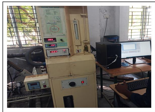
**Fig. 3: Setup of the single-cylinder DI diesel engine**
