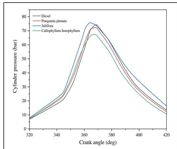
Fig. 15: Cylinder pressure with crank angle (deg)
