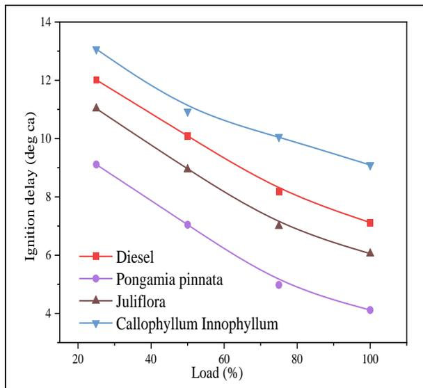
Fig. 17: Ignition delay with load (%)
