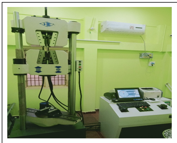
Fig. 3: UTM with fully automatic servo control
