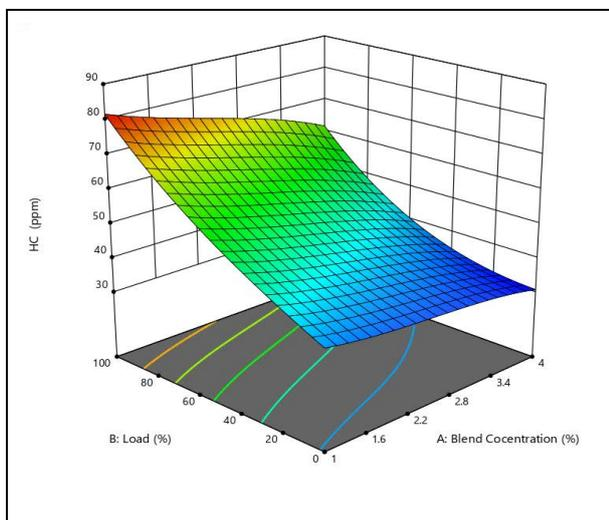
**Fig. 7: Variations of HC emission vs. Load**
