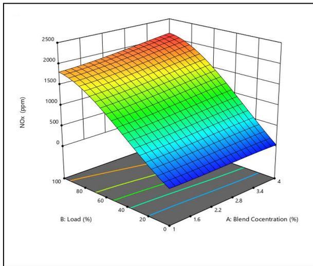
**Fig. 6: Variations of NO<sub>x</sub> emission vs. Load**
