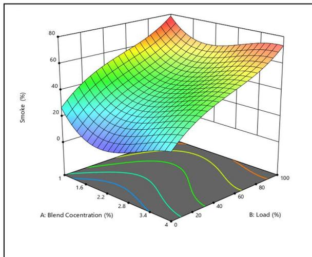
**Fig. 9: Variations in Smoke opacity vs. Load**
