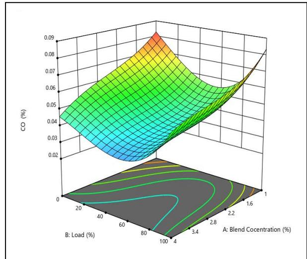
**Fig. 5: Variations of CO emission vs. Load**
