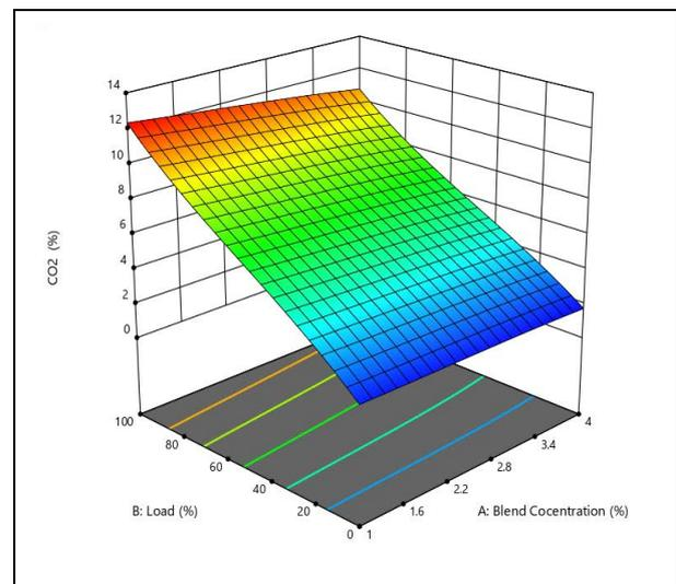
**Fig. 8: Variations in CO<sub>2</sub> emission vs. Load**
