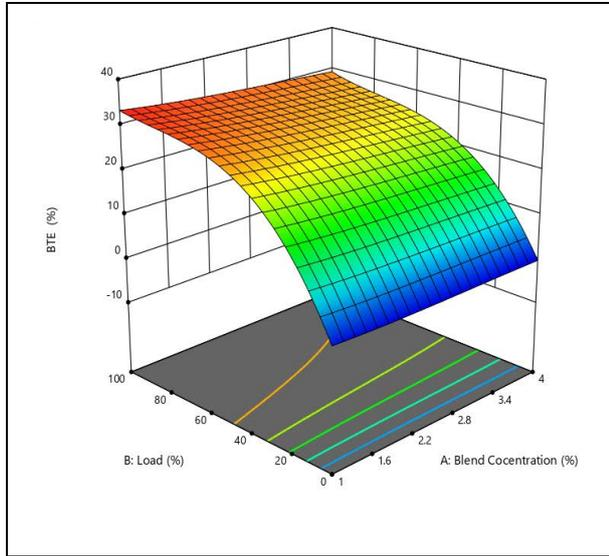
**Fig. 3: Variations of BTE vs. Load**
