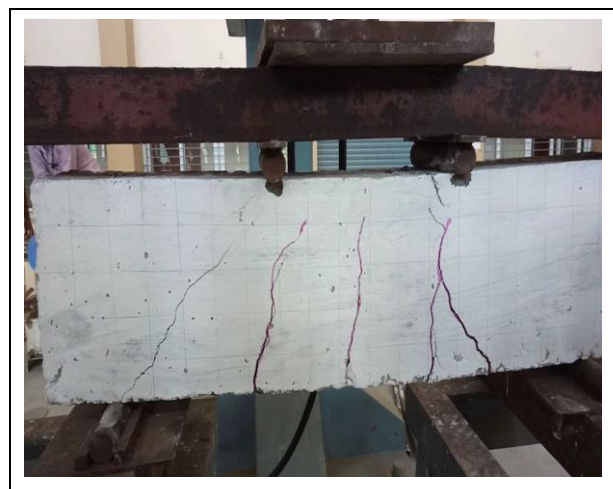
Fig. 1: RC Slab image using coconut fibers and Nano-SiO 2 .
