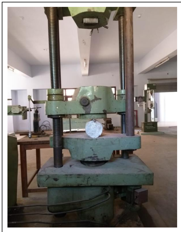
Fig. 3: Split tensile strength test
