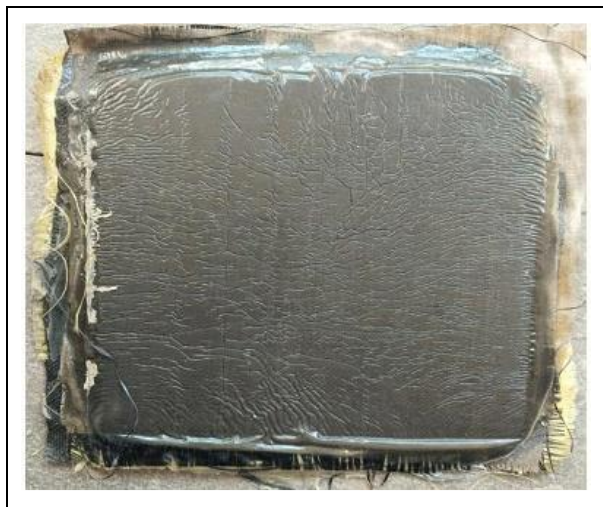
Fig. 6: Back view of 5 mm-thick cured composite
