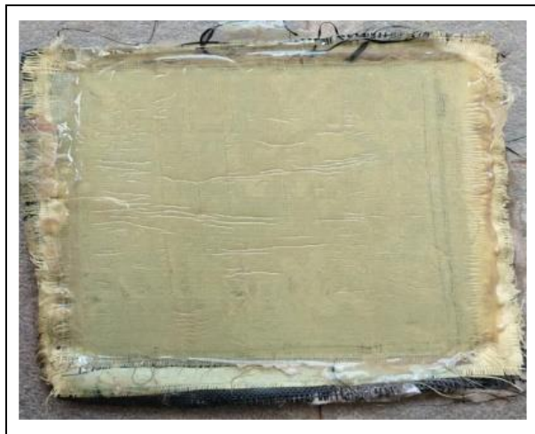
Fig. 5: Front view of 5 mm-thick cured
