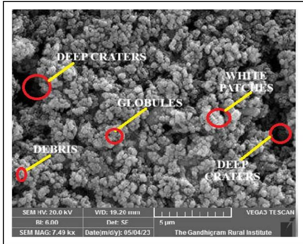
**Fig. 8: SEM image of aluminum nano ceramic powder**
