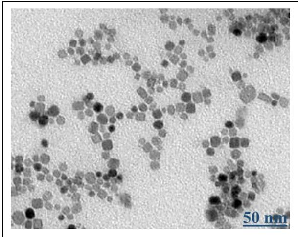
**Fig. 9: TEM image of aluminum ceramic powder**
