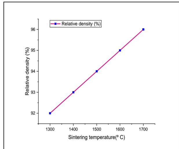
**Fig. 10: Relative density vs. sintering temperature**
