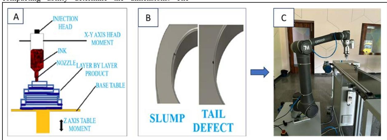
**Fig. 4:** DIW machine with issues of the samples and possible applications of DIW (a) DIW machine, (b) defect parts, and (c) Robotic arm (objective of our study)
