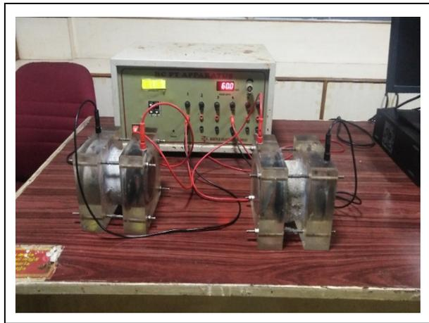
**Fig. 1: RCPT Test Bench**
