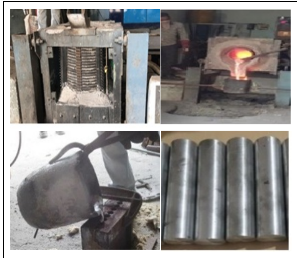
Fig. 1: Electromagnetic stir casting setup
