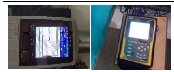
Fig. 11: Surface roughness tester and power quality analyzer
