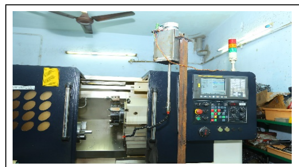
Fig. 8: CNC setup with solid lubrication supply system
