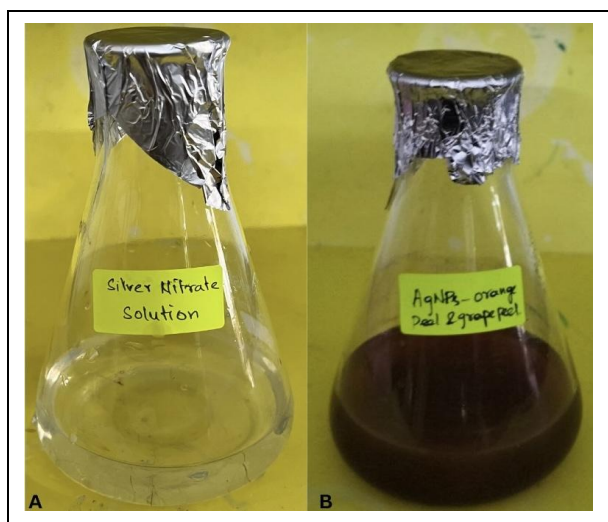
Fig. 3: Preparation of chitosan-AgNPs
