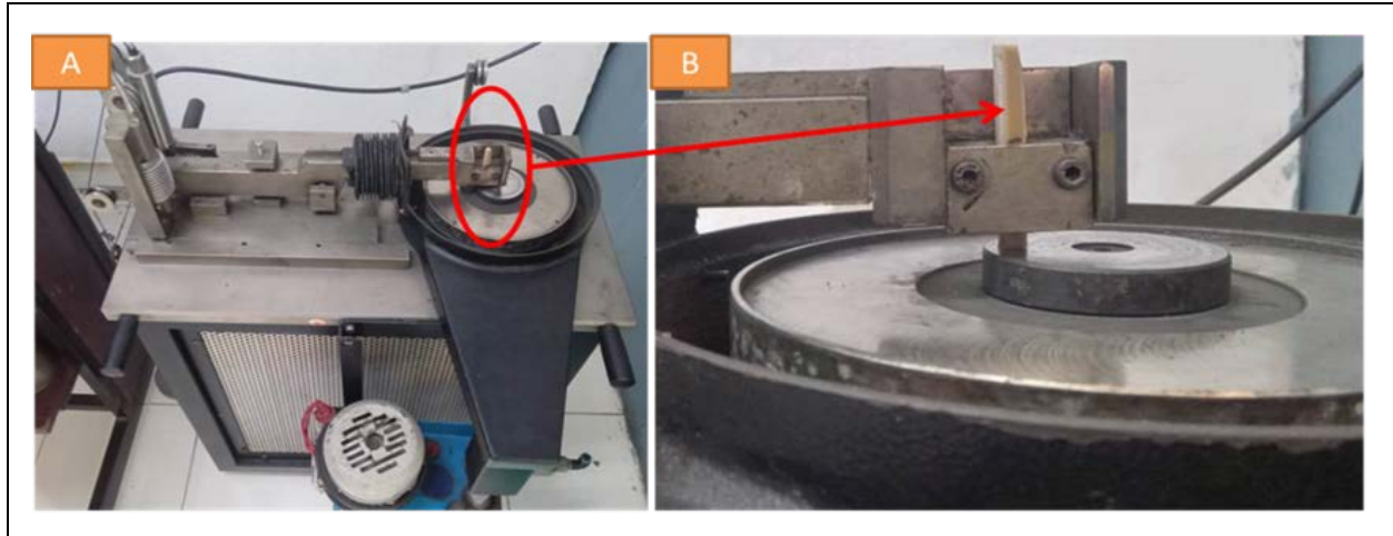
Fig. 1: Pin-on-disc (a) machine setup (b) enlarged view of sample position
