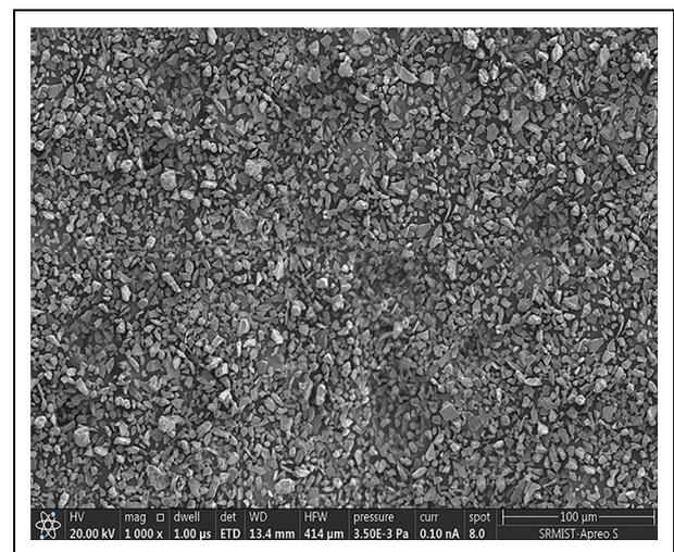
Fig. 2: SEM Image of alumina nanoparticles
