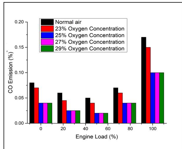
Fig. 4: Engine load (%) vs CO emission (%)
