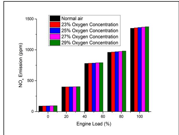
Fig. 7: Engine load (%) vs NO<sub>x</sub> emission (ppm) with nanoparticle addition
