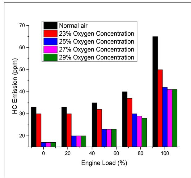
Fig. 3: Engine load (%) vs HC emission (ppm)
