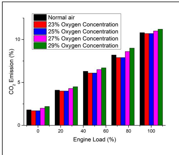
Fig. 5: Engine load (%) vs CO<sub>2</sub> emission (%)
