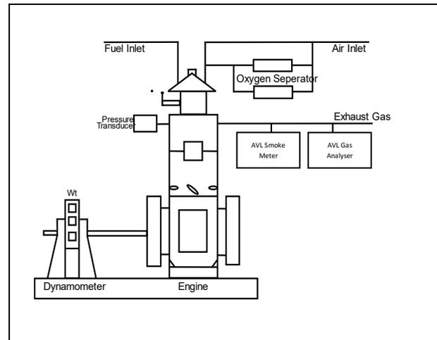
Fig. 1: Test engine setup
