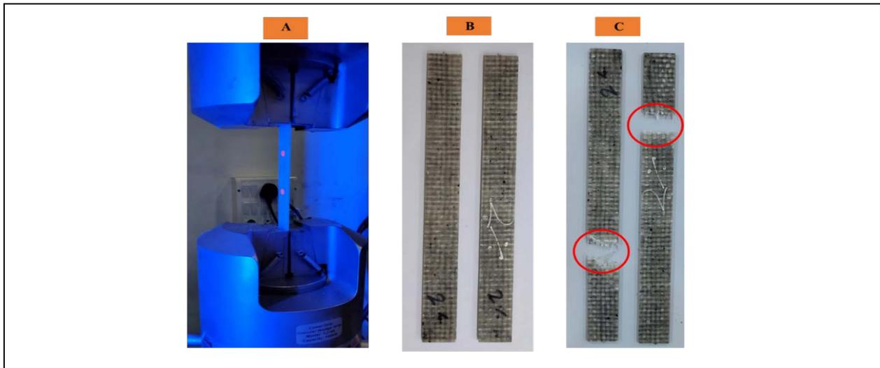
Fig. 1: Tensile test setup with specimen with and without failure
