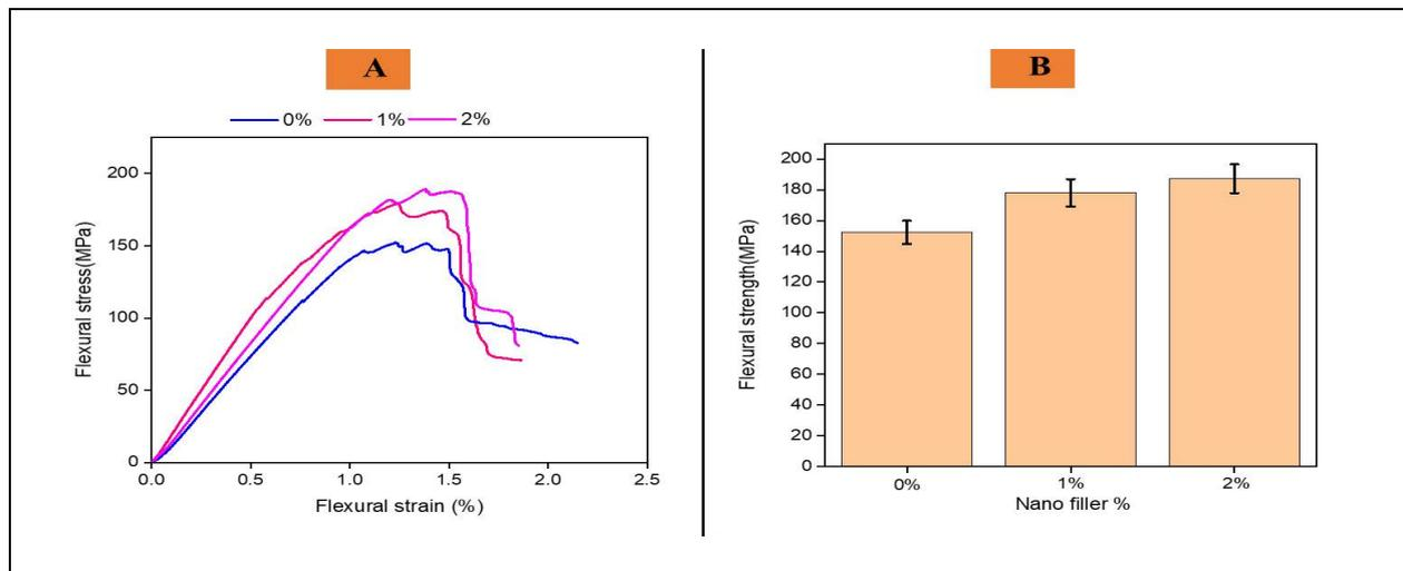
Fig. 4: A: Flexural stress-strain curve for samples with 0%, 1%, and 2% nanomaterial concentrations. B. Data shown as bar graph
