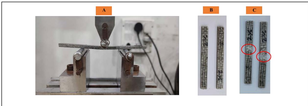
Fig. 2: Three-Point bending test setup with specimen with and without failure
