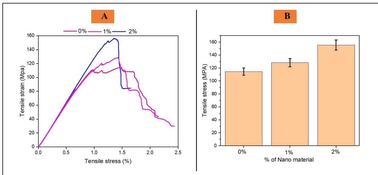
Fig. 3A: Tensile stress-strain curve for samples at 0%, 1%, and 2% nanomaterial concentrations B. Data shown as bar graph
