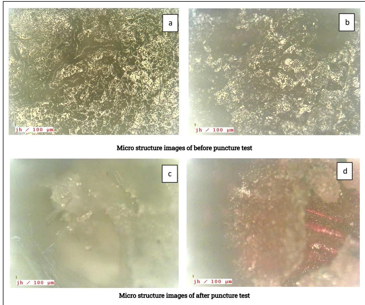
**Fig. 8. The microstructure view of jute composite**
