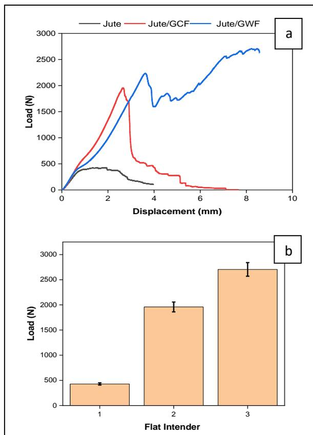
**Fig. 5. Load vs Displacement and, illustrating error bar of the composites of flat intender**
