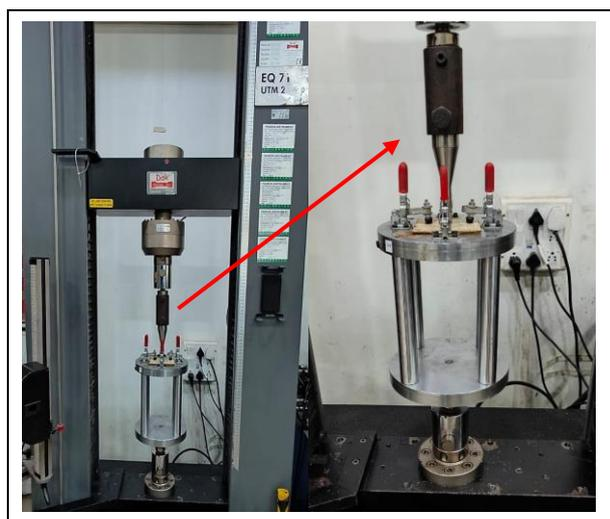
**Fig. 3. A and B is Setup for the Puncher Test using a universal testing machine and Shows a closer view of the testing jig or fixture**
