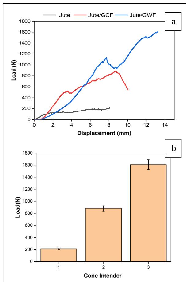
**Fig. 6. Load vs Displacement and, illustrating error bar of the composites of cone intender**
