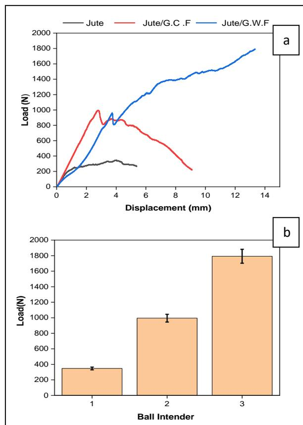
**Fig. 7. Load vs Displacement and, illustrating error bar of the composites of ball indenter**
