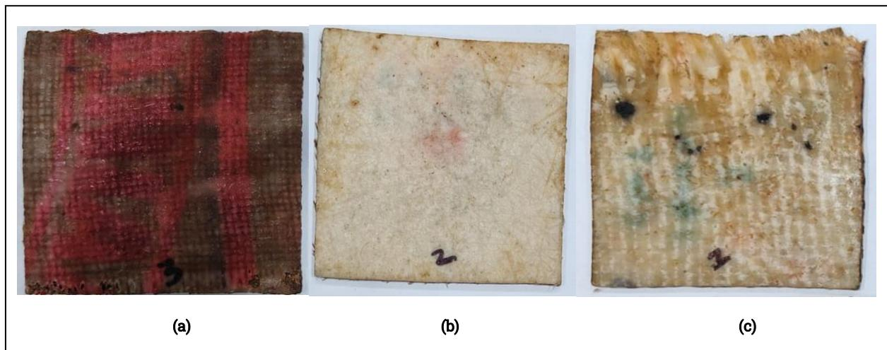
Fig. 1. Schematic representation of the materials: (a) Jute (b) Glass carbon fiber (c) Glass woven fiber
