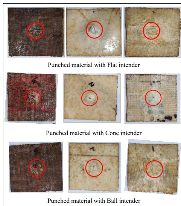
**Fig. 4 . Materials after the impression of the Ball Indenter Jute, Glass Carbon Fiber, and Glass Chopped Fiber, along with Ball Indenter Setup**
