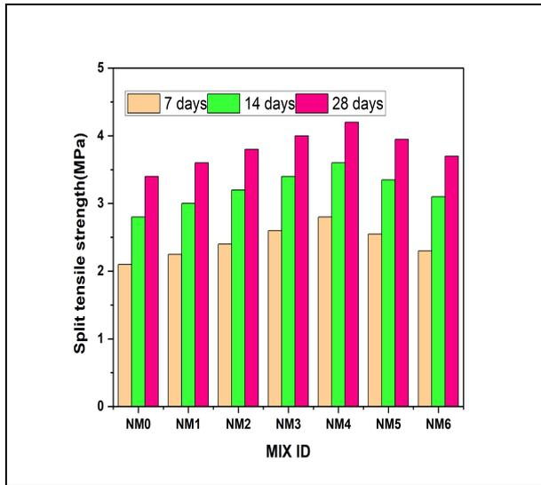
Fig. 4: Test findings of Split Tensile Strength for Various SCC Mixes
