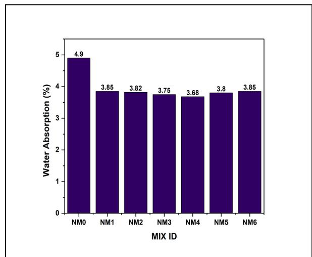
Fig. 6: Water absorption of SCC mixes
