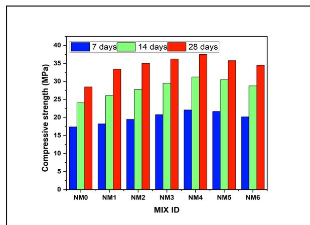
**Fig. 3: Test findings of compressive strength for various SCC mixes**
