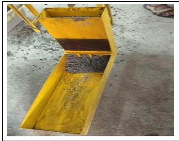
Fig. 2(a): L-box test
