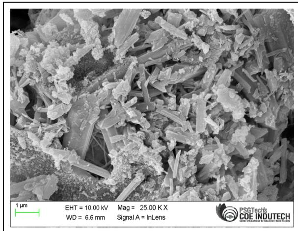
**Fig. 7b: SEM photograph for conventional mix**
