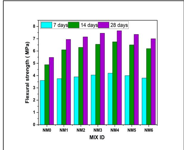
Fig. 5: Test findings of flexural strength for various SCC mixes
