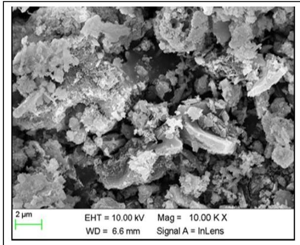
**Fig. 7a: SEM photograph for NM4 concrete blend**
